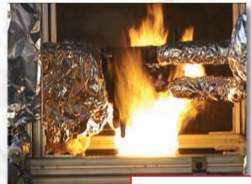
Aircraft engine component being subjected to fire test
