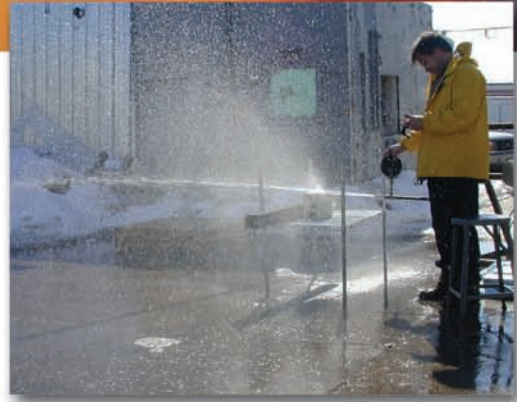
Waterproof test performed on electronic enclosure
