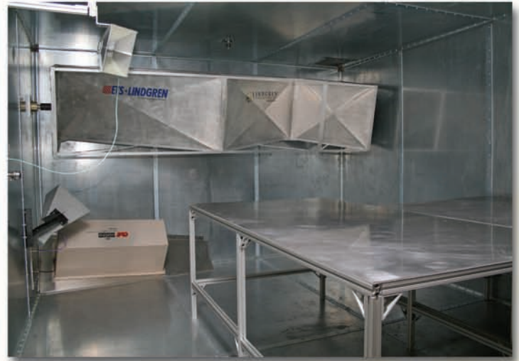
HIRF/Mode tuned chamber
