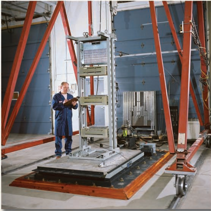
Zone 4 earthquake test from GR-63-CORE performed on hydraulic shaker
