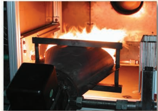
Aircraft engine component subjected to fire test
